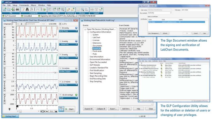
Above: The GLP Client adds a GLP Status Bar to the LabChart application window and an Audit Log (right panel) that records the user, GLP status, configuration and recorded data information.
