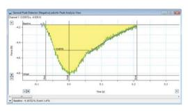
Peak Analysis View displaying a negative peak and its parameters.
