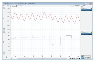
Breath temperature is measured on the top channel using the Thermistor Pod. The breathing rate is calculated from this and displayed on the second channel.
