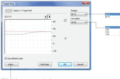
Click this button to view or alter the calibration of the T-type thermocouple.
